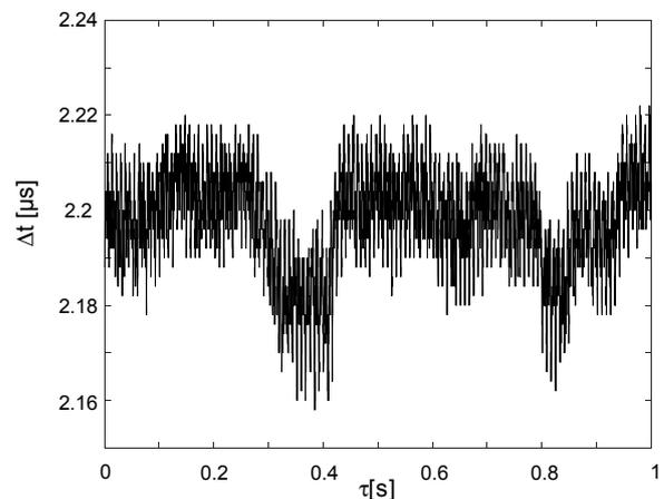
**Figure 2. Time sequence of the realized laser pulse separation  $\Delta t$  for an assigned  $(\Delta t)_a = 1.6 \mu\text{s}$ .**
