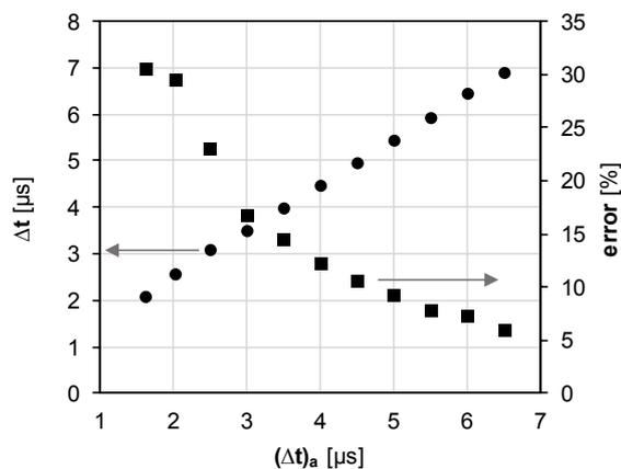
Figure 3. Mean realized laser pulse separation  $\Delta t$  (●) with the assigned  $(\Delta t)_a$  and the corresponding error (■).
