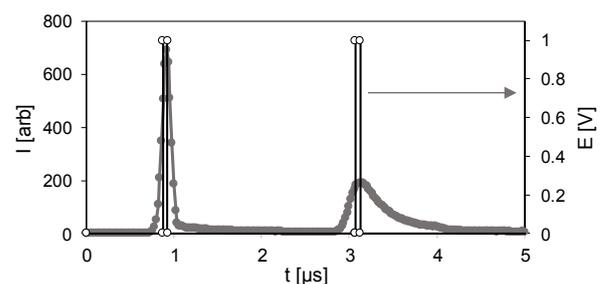
Figure 4. Light intensity of the laser double-pulse captured by the photodiode and the corresponding output of the circuitry described in section 2.2.
