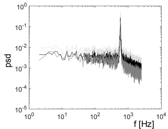
**Figure 5. Power spectra of the velocity fluctuations measured by the HWA (dark grey) and the uncorrected (light grey) and corrected (black) PIV measurements.**
