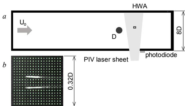
**Figure 1. Experimental setup (a) and the zoomed-in PIV measurement plane with overlaid hot wire sensor (b).**
