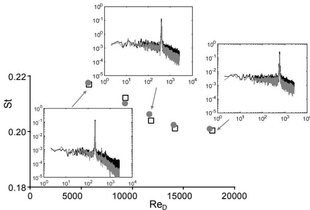
**Figure 6. Strouhal number of the cylinder wake with Reynolds number measured by the HWA (circle) and PIV (square), and three characteristic pairs of spectra of the velocity fluctuations (HWA in dark grey, PIV in black).**
