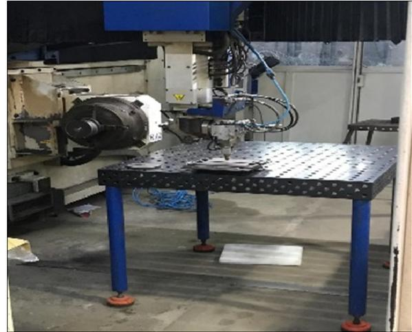
Figure 1. (a) CO<sub>2</sub> Laser welding machine
