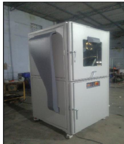
Fig.12. Manufactured dust test chamber
