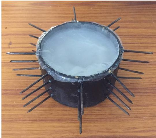
Figure 4. Photograph of finned cup with wax covered with LLDPE
