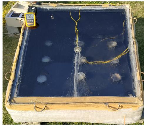
Figure 6. Photograph of finned cup with wax covered with LLDPE
