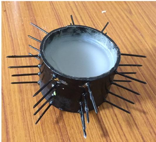
Figure 3. Photograph of finned cup with wax
