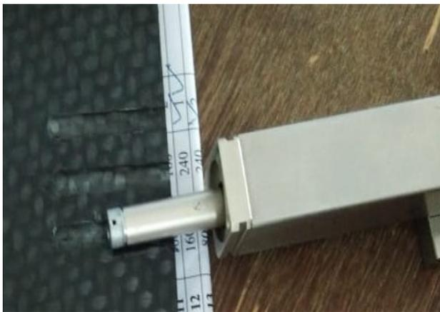
Figure 2. Surface roughness setup
