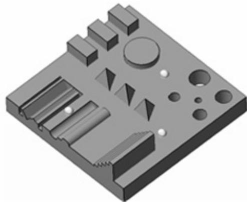
**Figure 3. Benchmark part with three similar spheres for establishing common reference system**
