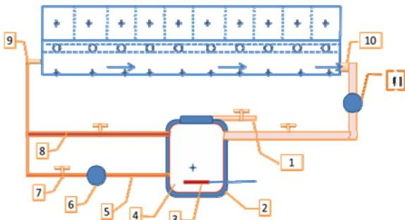
1. Inlet to the storage tank, 2. Thermal insulation of the tank, 3. Electrical water heater 4. Water 5. Feed pipeline to the electric pump, 6. Water pump 7. Control valve, 8. pipeline for the recirculation, 9. Feed pipeline to the long still, 10. Discharge pipeline of long still, 11. Hot water flow meter,  $\uparrow$  Thermocouples
