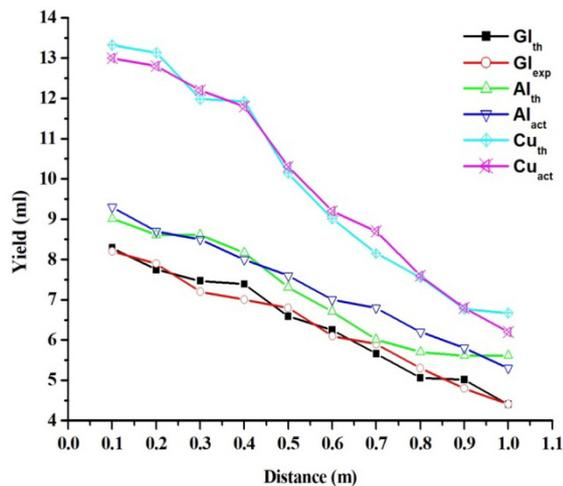
**Figure 7: Variation of the experimental and theoretical distillate output from the long stills covered with *GI*, *Al*, and *Cu* sheet material along the length.**
