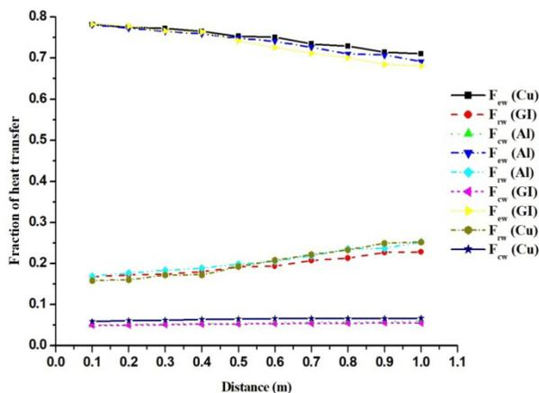
**Figure 8: Variation of the fraction of heat transfer along the length of the long stills**
