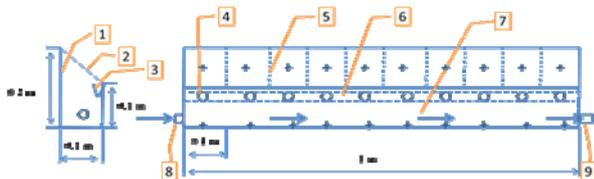
1. Basin of long still, 2. Al/Cu/GI sheet covers of 4 mm thick plate 3&6. Condensate gutter, 4. Drain to collect distillate yields from ten equidistance locations, 5. Partition of the Al/Cu/GI sheet, 7. The flow direction of hot wastewater 8. Inlet of the long still, 9. An outlet of long still,  $\uparrow$  Thermocouples
