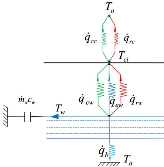
Figure 3(b) Thermal circuit of long still
