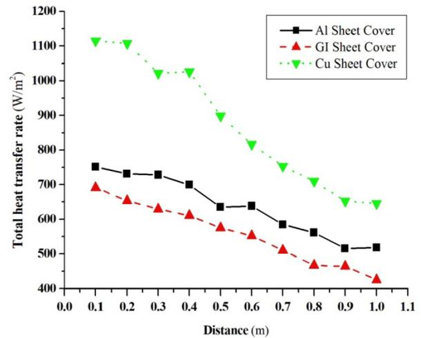
**Figure 6: Variation of the total heat transfer rate of long stills with different metallic cover as a function of time.**
