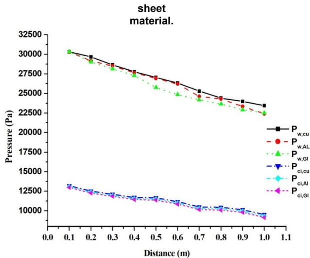
**Figure 4: Variation of the partial pressure on the water surface and condensation surface of *Cu*, *Al*, and *GI* sheet cover material along the length of the still.**
