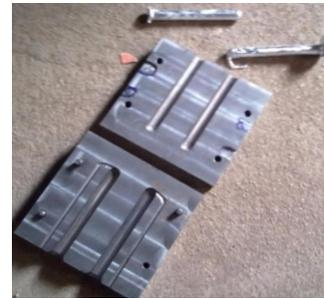
Figure 1. Permanent mold for producing composites.
