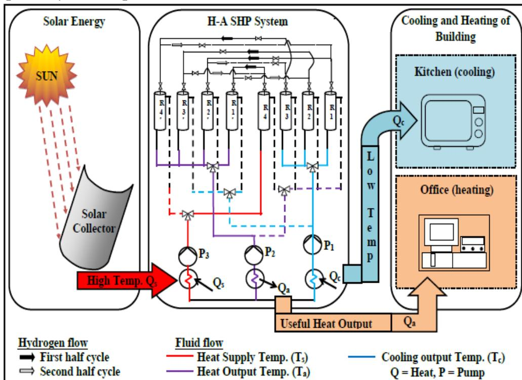
Figure 1. Schematic of multi-stage sorption heat pump for building air-conditioning [10]
