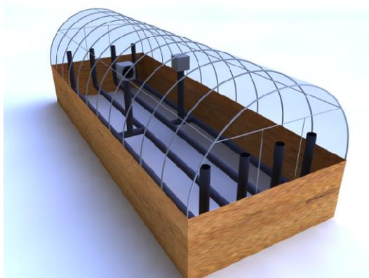
**Figure 3. A rock-bed heating system in a greenhouse**
