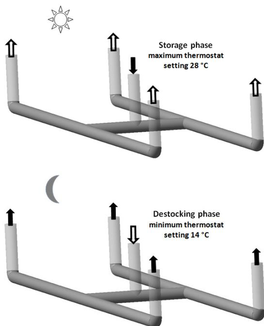
Figure 5. Operating principles of the rock-bed heating system
