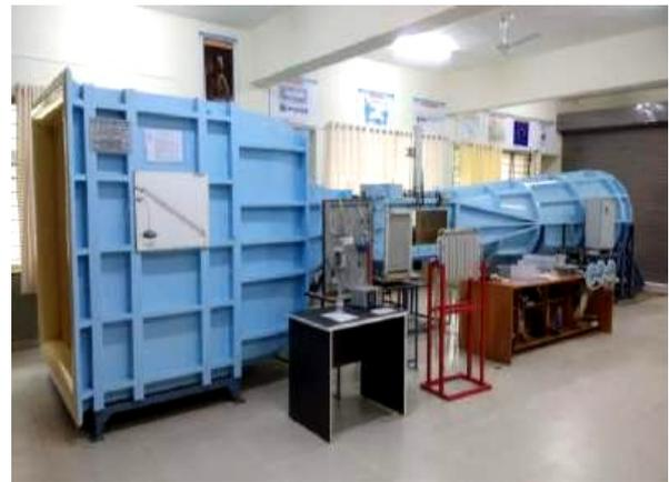
Figure 4. Photograph of the subsonic wind tunnel used in the present investigation.
