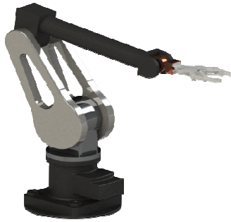
Figure 3. The adopted robotic system with 3 DOFs
