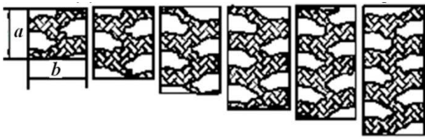
Figure 3. A change in the dimensions of the wheel-to-ground contact depending on the normal load
