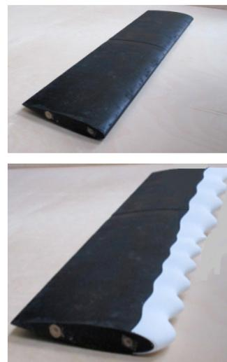
**Figure 1. Overview of the experimental blades, the normal blade (up) and wavy blade (down).**
