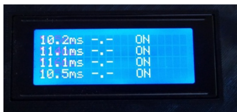
Figure 8. Fuel injection time control on the display of the DBD-4 device
