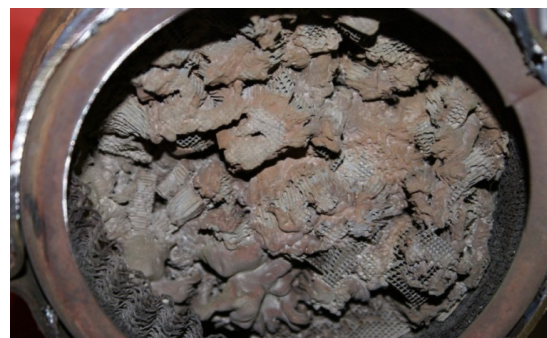
Figure 2. A catalytic converter with an irreversible change in the internal cells of the catalytic part
