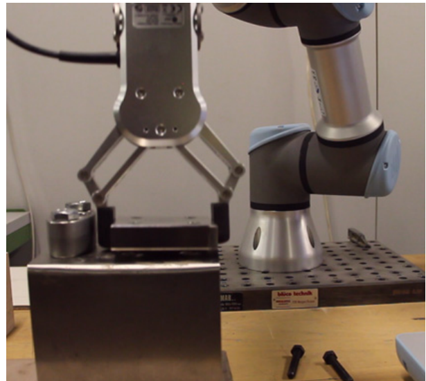
Figure 6. Robot mounts the square flange on the base by executing a task-oriented program after receiving the indication of the target position by the operator
