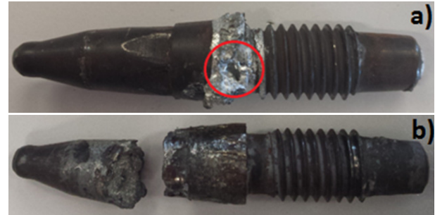
Figure 2. External aspect of some nozzles removed from the high-pressure die-casting equipment after severe damage: (a) exhibiting a hole; (b) or even being broken
