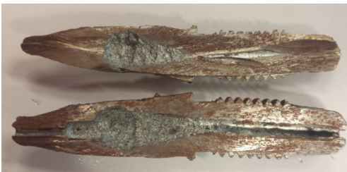
Figure 5. Sample 2 - Wear sustained by an injection nozzle (original design) after 17 days of use, at an injection rate of 500 injections per hour.
