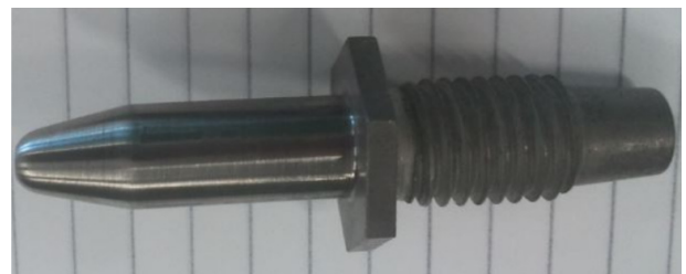
Figure 16. Chosen design for the injection nozzle (second iteration).
