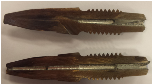
Figure 9. Sample 2 – Wear sustained by injection nozzle (first iteration) after 47 days of use, at an injection rate of 500 injections per hour.
