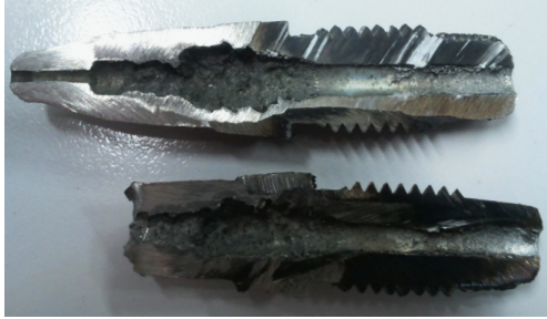
Figure 4. Sample 1 - Wear sustained by injection nozzles (original design) after 11 days of use, at an injection rate of 500 injections per hour.
