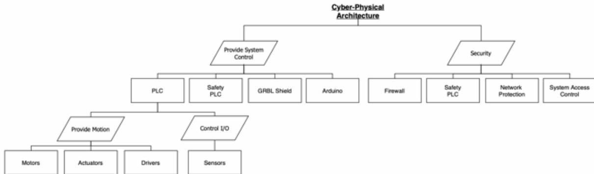
Figure 9. Function Means Analysis (Cyber Physical)
