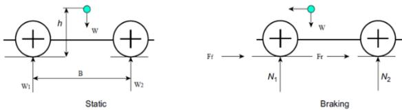
**Figure 2. Dynamic effect on the vehicle during the static and braking conditions**
