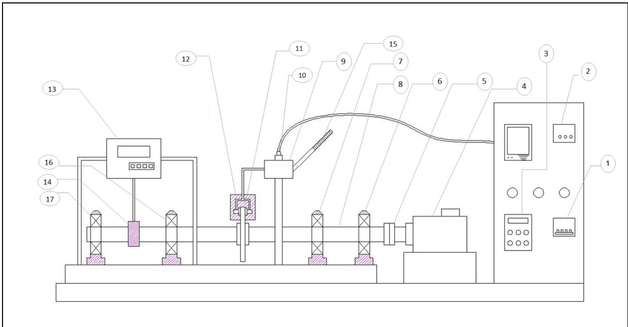
**Figure 7. Schematic Diagram of Disc brake set-up.**
