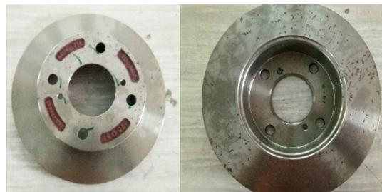
**Figure 9. Brake Disc (Rotor Disc)**
