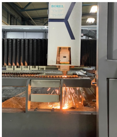
Figure 1. Example of cutting by fiber laser.
