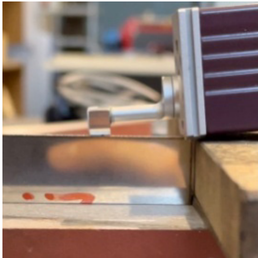
Figure 6. Measurement of specimen roughness.
