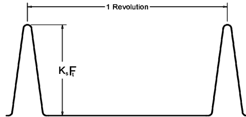
Fig. 1a: Pulsating bending load
