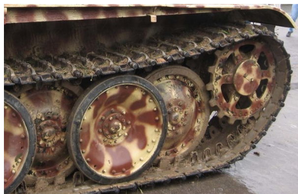
Figure 3. Caterpillar undercarriage system with staggered track wheels
