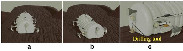
**Figure 4. Scenes of the movement of a mobile robot along a tree trunk: a – the rectilinear movement of the robot; b – rotation of the robot when changing the movement route; c – taking laboratory samples of wood with a drill tool.**
