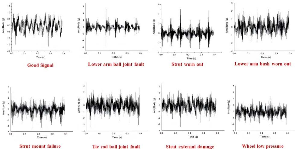
**Figure 4. Sample of vibration plots of suspension conditions**
