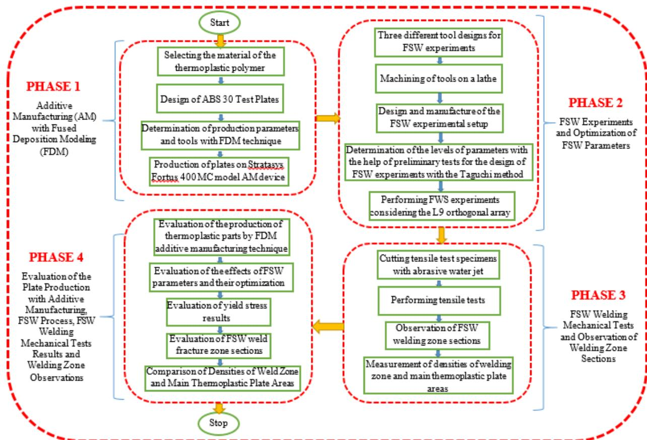
Figure 2. Flow chart of the experimental study
