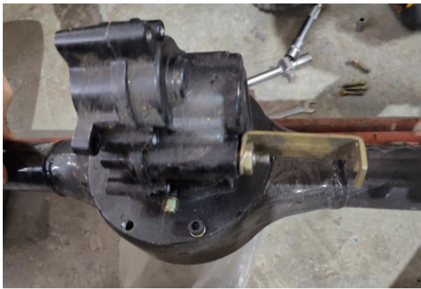
Figure 5. Two-speed gearbox with differential
