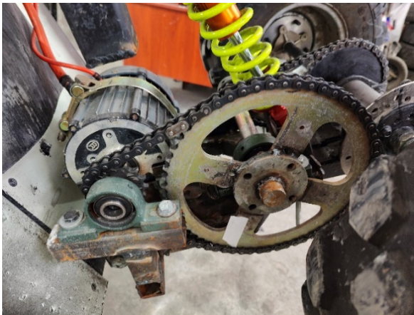
Figure 3. Two-stage chain, front view
