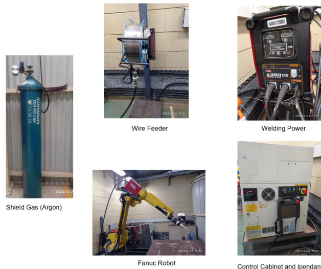
Figure 1. Welding robot system in the experiment
