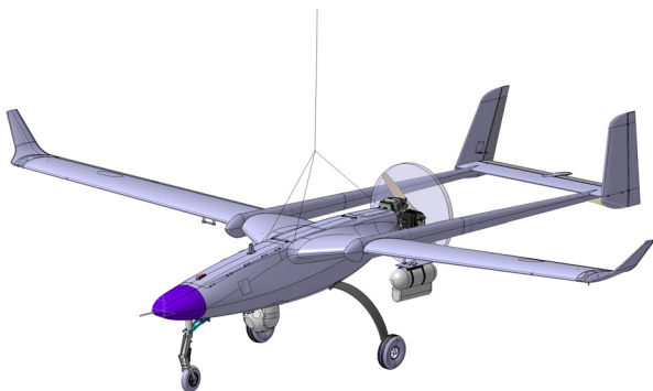
Figure 4. OUT unit attached to the wing pylon
