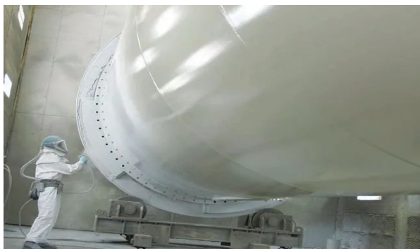
Figure 8. Wind Turbine Blade Coating Process [25].
