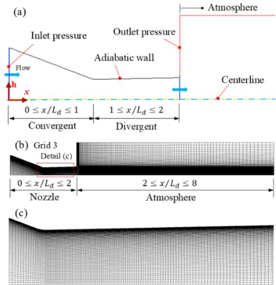
**Figure 3. (a) 2D computational domain, showing the boundary conditions in the nozzle and in the atmosphere. (b) Grid 3 with 26385 quadrilateral cells. (c) Enlarged detail of the mesh of the divergent nozzle.**
