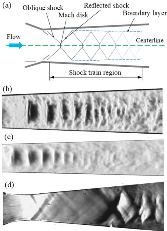
**Figure 1. (a) Illustrative basic schematic of the shock train structure in the divergent for a very narrow angle nozzle [19]. (b) and (c) Shock train in a divergent duct reported by Weiss et al. [16] and, (d) reported by Matsuo et al. [4].**
