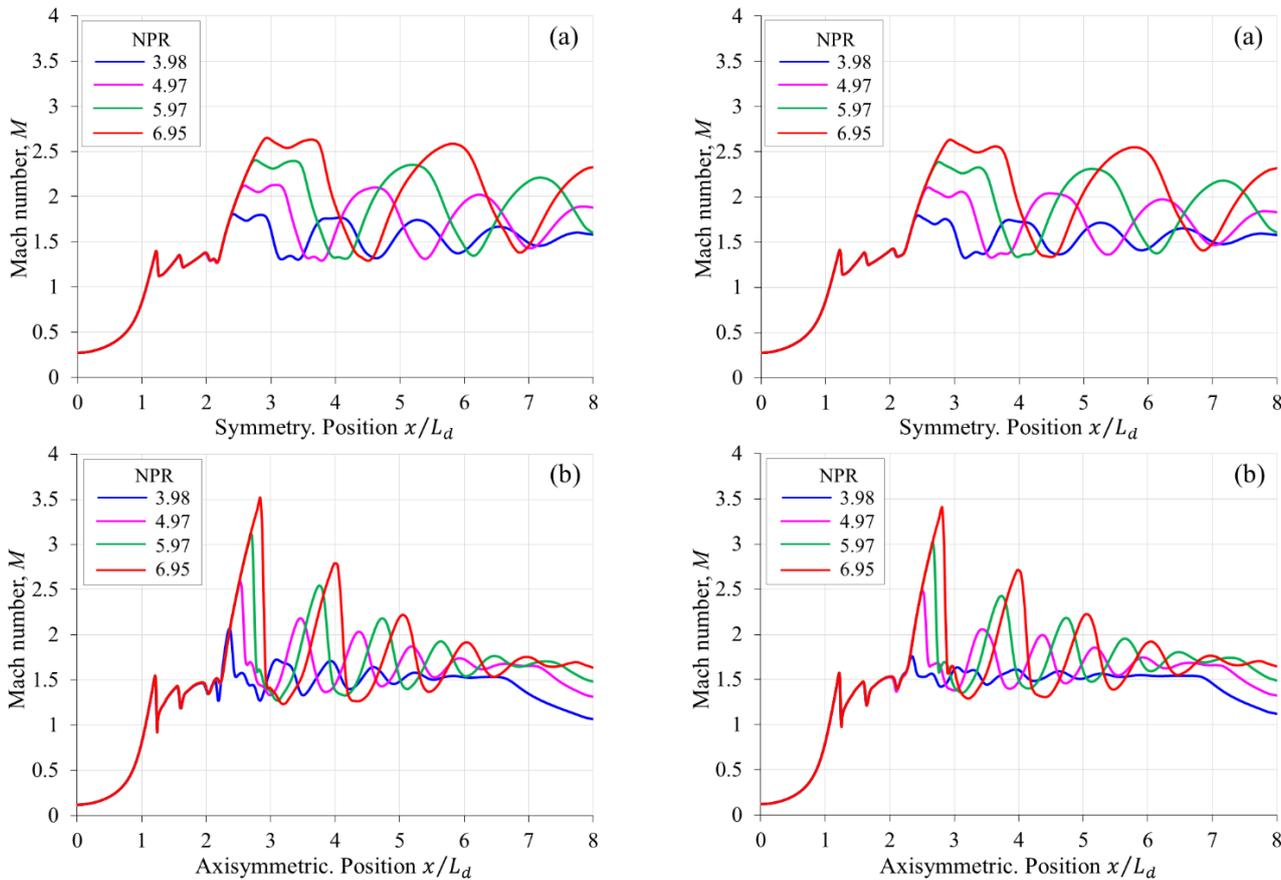
Figure 9. Mach number profiles on the centerline for the divergent with  $\alpha = 1^\circ$ : (a) Planar nozzle and (b) Conical nozzle.
