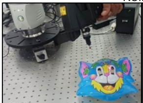
c. Laser scanning of the mask.
