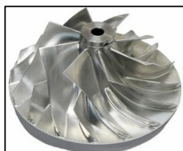
b. 05-axis machining.
