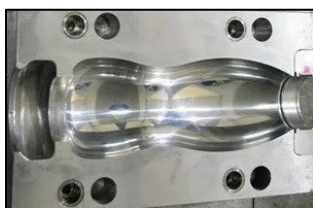
a. 03-axis machining.
