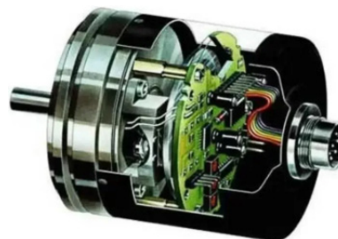
Figure 1. An optical rotary encoder [8]
