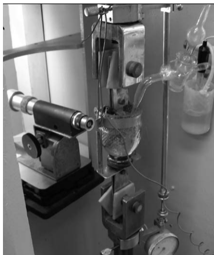
Figure 2. Photo of electrochemical cell for SCC research.
