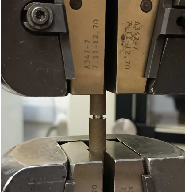
Figure 3. Experimental setup for tensile test
