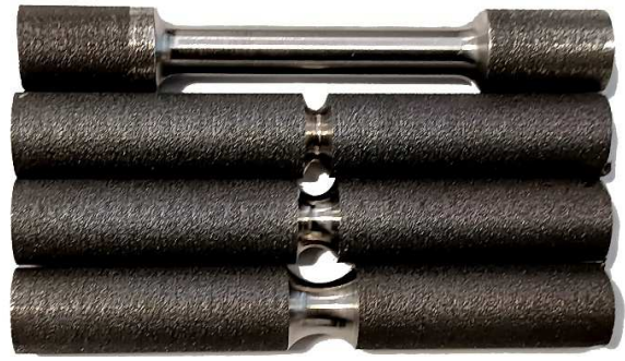
Figure 1. Machined tensile test specimens
