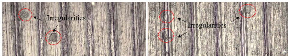
Figure 12. Machined surface texture observed by optical microscope Eclipse LV150N Nikon at X10 magnification
